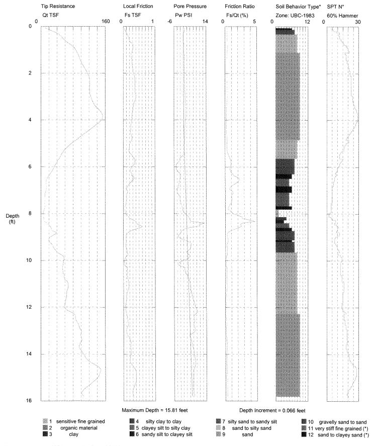
Operator: WATKINS Sounding: C-3 Cone Used: DSG1034 Groundwater Level: 4.3 feet CPT Date/Time: 4/10/2008 2:27:41 PM Location: Vanguard Bank, Panama City, FL
