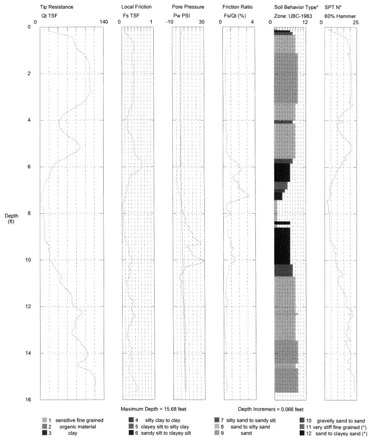
Operator: WATKINS Sounding: C-2 Cone Used: DSG1034 Groundwater Level: 4.2 feet CPT Date/Time: 4/10/2008 3:04:51 PM Location: Vanguard Bank, Panama City, FL
