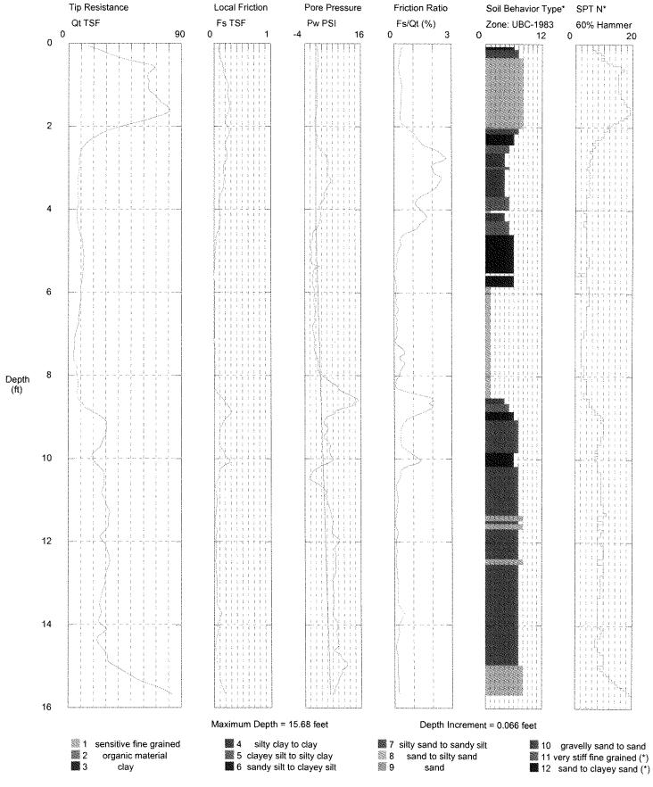
Operator: WATKINS Sounding: C-4 Cone Used: DSG1034 Groundwater Level: 3.8 feet CPT Date/Time: 4/10/2008 2:39:41 PM Location: Vanguard Bank, Panama City, FL
